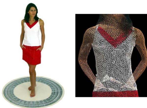
Figure 4: Scanning with digital Body Capture System "*BodySABA 0.3.*" and digital 3D presentation of the object scanned in Wireframe
