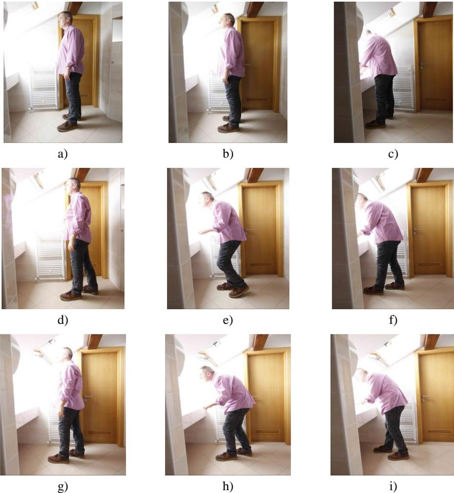
**Figure 2.** Access zones for a person with a window sloped to 210 cm (a, b, c), 190 cm (d, e, f) and 170 cm (g, h, i)
