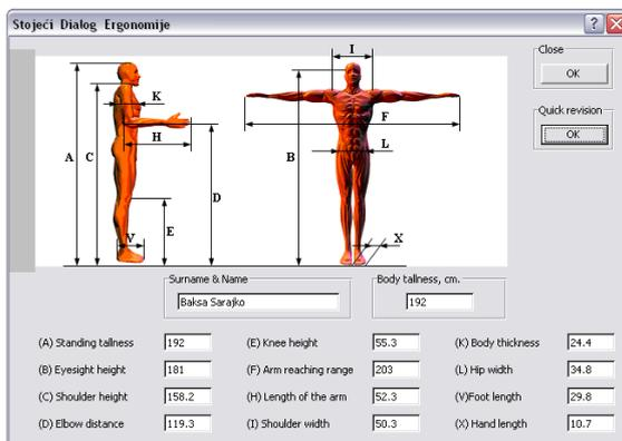
**Fig. 5.** On-screen presentation of characteristic anthropometric measures for a standing male person
