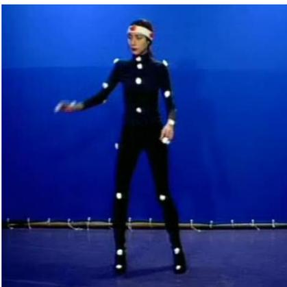
**Fig. 9.** *Studio recording with VatoSABA 1.4. motion capture system*
