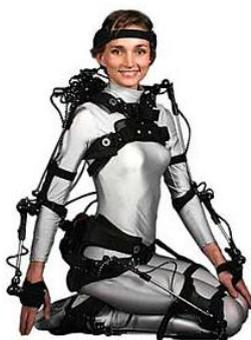
**Fig. 7.** *Gypsy motion capture system*
